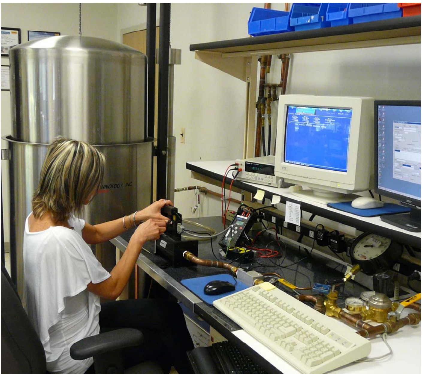
Bell prover used by technician in calibrating high flow capacity flow meter.
